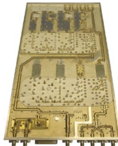
RF Distribution Network
