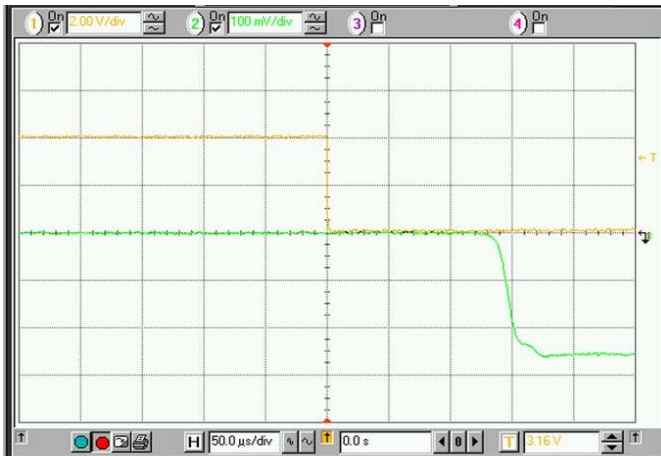
Switching time RF Off (TTL 1) to RF ON (TTL 0) (Yellow - TTL, Green - RF signal)
