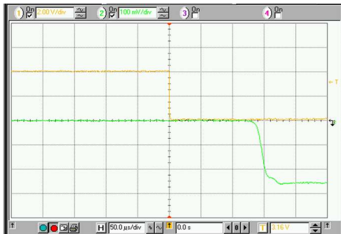
Switching time RF Off (TTL 1) to RF ON (TTL 0) (Yellow - TTL, Green - RF signal)
