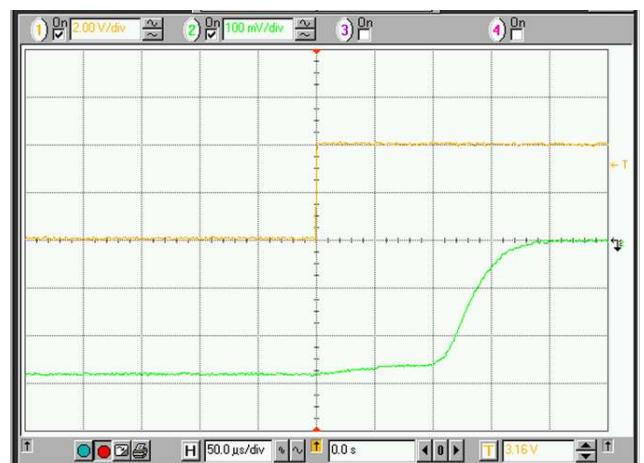
Switching time RF On (TTL 0) to RF Off (TTL 1) (Yellow - TTL, Green - RF signal)
